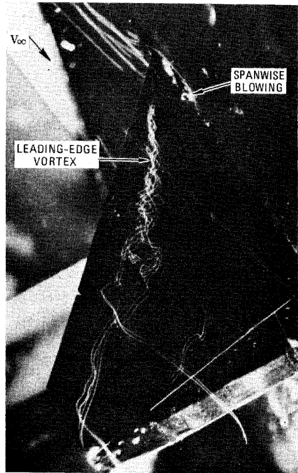
Fig. 3 Spanwise blowing on a 44 deg swept trapezoidal wing; \alpha = 20 deg (from Ref. 1).
